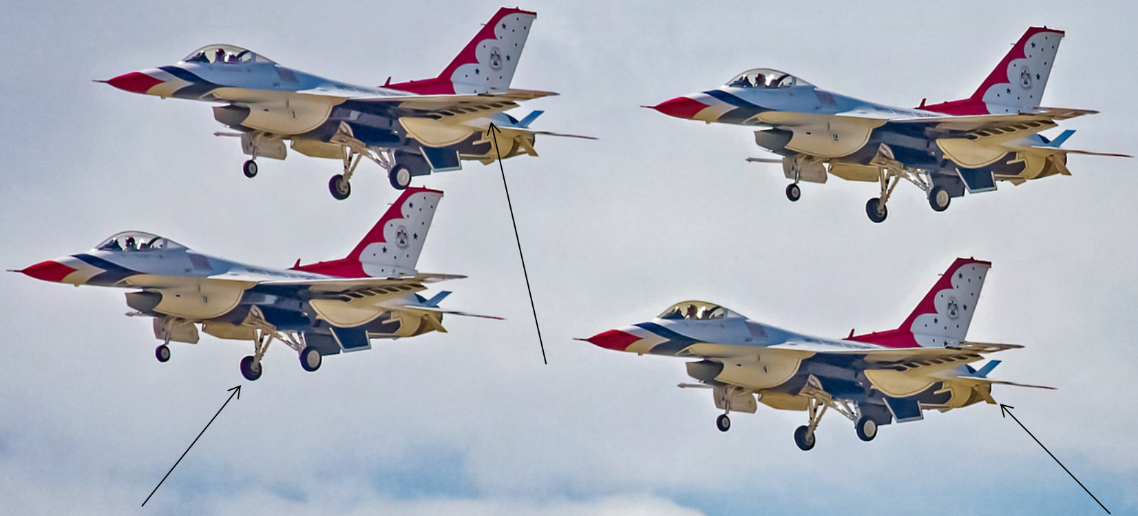
Aircraft performance demo – “dirty configuration” Landing gear, flaps and air brakes all deployed
